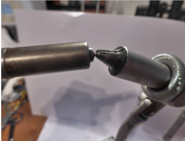
Fly tying vice to pull the internal out enough to remove the circlip
