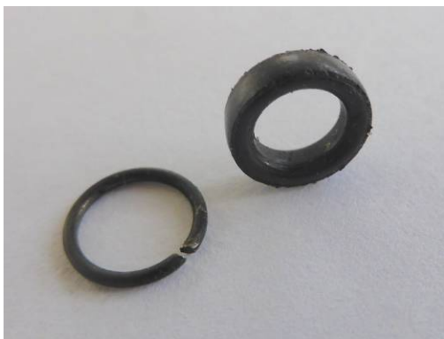
Original O-ring and circlip.
